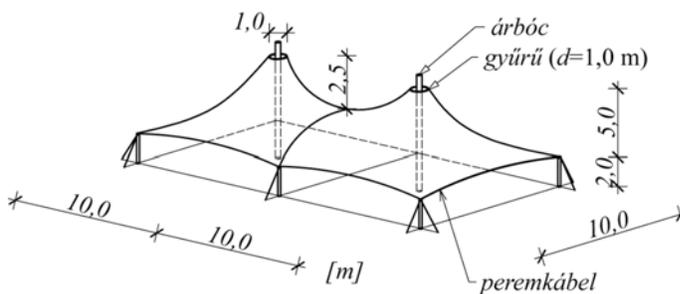
The second exercise presents another possibility for pre-tensioning: the usage of hyperbolic surface. The internal forces of the two-mast-supported tent structure can be exactly determined only by nonlinear finite element method, however, the discussed simplifications and considerations make the manual calculations suitable.
