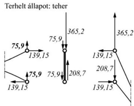
The tensioned foundation is verified in two cases: First, the self-weighted foundation, that transmits the loads to the soil, which is a plastic material without tensile strength. This balances the foundation against the normal forces and moment caused by the columns and cables. In the second case long enough soil anchors are applied that transmit the tension to the lower layers of the soil.
