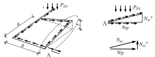
$$\overline{N_{xy}} * f * 2 = p_{Ed} ab = 4,28 * 5 * 6 = 128,4 \text{ kN}$$
