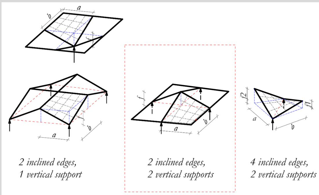
Both internal forces and support reaction forces can be determined based on the method shown above, even, if  $a$  differs from  $b$ . Hence each can be expected at TEST 2.
