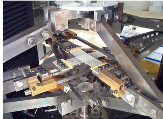
Fig. 3. Biaxial tensile device on cross shape specimens.
