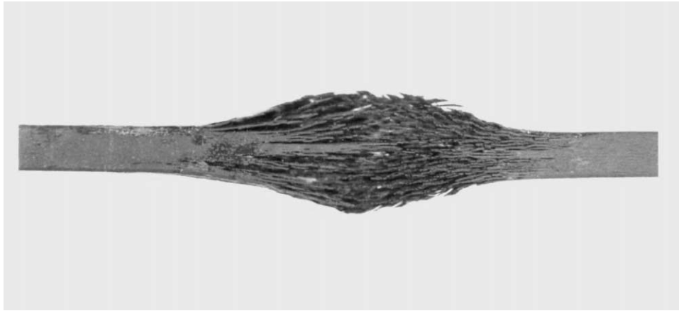
Fig. 3. Side view of a tested 8HS woven graphite/PMR-15 off-axis specimen showing interlaminar delaminations after unloading.
