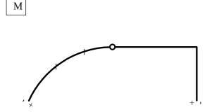
5. Determine the internal force diagrams of the following structure if its shape is the graph of the function y=bx<sup>2</sup> (parabola)! The heights of the points from axis x are denoted by  $h_1$ ,  $h_2$ ,  $h_3$ , the angles between the tangents of the parabola and axis x are denoted by  $\alpha_1$ ,  $\alpha_2$ ,  $\alpha_3$  (see the figure below). The force in the tie rod is denoted by S. The heights are required in centimeters! (10 + 10 points)
